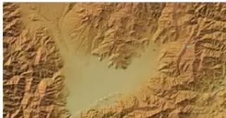
The neat thing about is that it is the **most precise global-scale elevation data** now. It uses the Advanced Land Observing Satellite "DAICHI" (ALOS) based on stereo mapping from PRISM.
